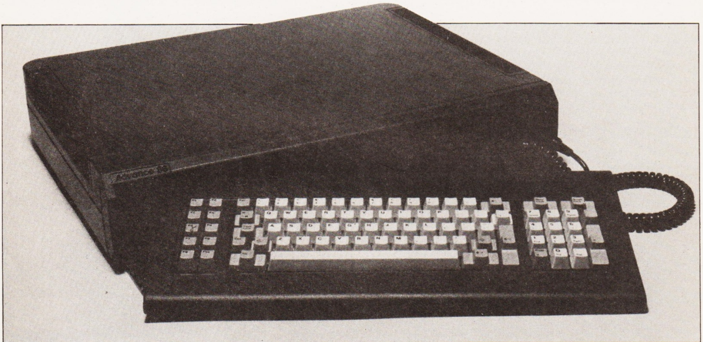
The keyboard slides inside the main casing when not in use.
