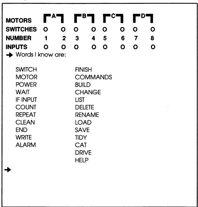
For your convenience all the red function keys have been designated as a command word. A function key strip is provided with this manual and should be inserted under the hood of the BBC computer. Thus pressing <f0> will type for you the command words SWITCH ON followed by the necessary space. The function keys are as follows:
