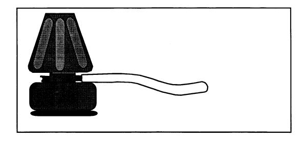
Screw down the plastic top of the post to secure the wire in place. this will ensure a good electrical contact.
