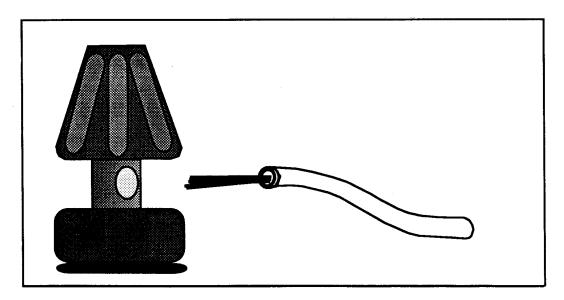
To connect a bare wire to the control box simply unscrew the post mounted on top of the box and thread the wires through the hole.
