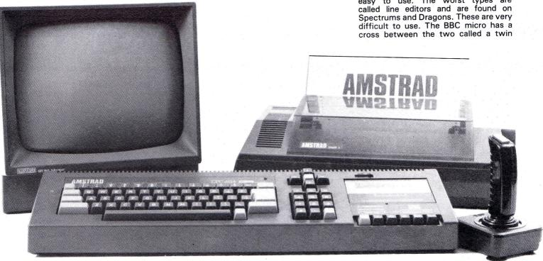
television - in fact the tube is a standard TV tube and doesn't give the definition of a dedicated RGB monitor. It can just about resolve 80 columns, but not very well. The 80 column mode of the Amstrad can get quite tiring on the eyes with the colour monitor.
