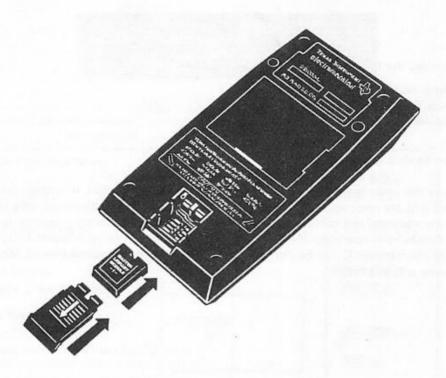
Don't touch the contacts inside the module compartment as damage can result.
