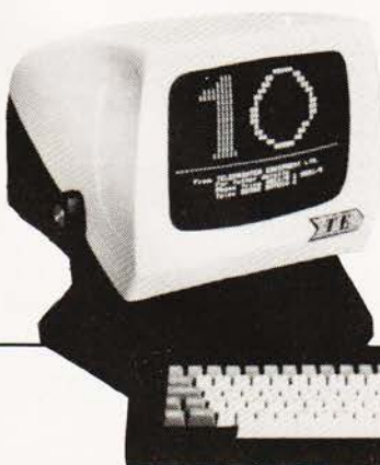
The Teleray Model 10, one of a three series range of micro-processor controlled VDU terminals.
