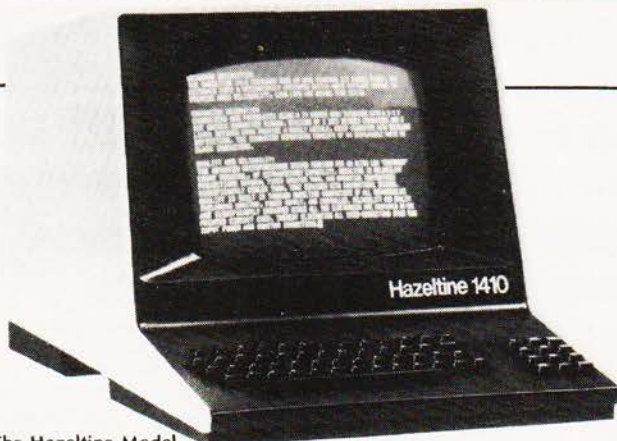
The Hazeltine Model 1410 with 'no frills' VDU.
