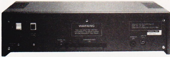
Left: The rear panel of the MC. The cassette and serial ports share a single connector.
