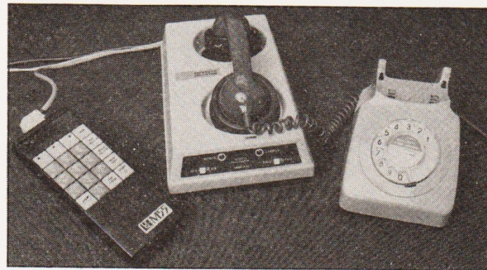
A typical setup: Selecta Keypad, Modem/acoustic coupler and...a telephone.
