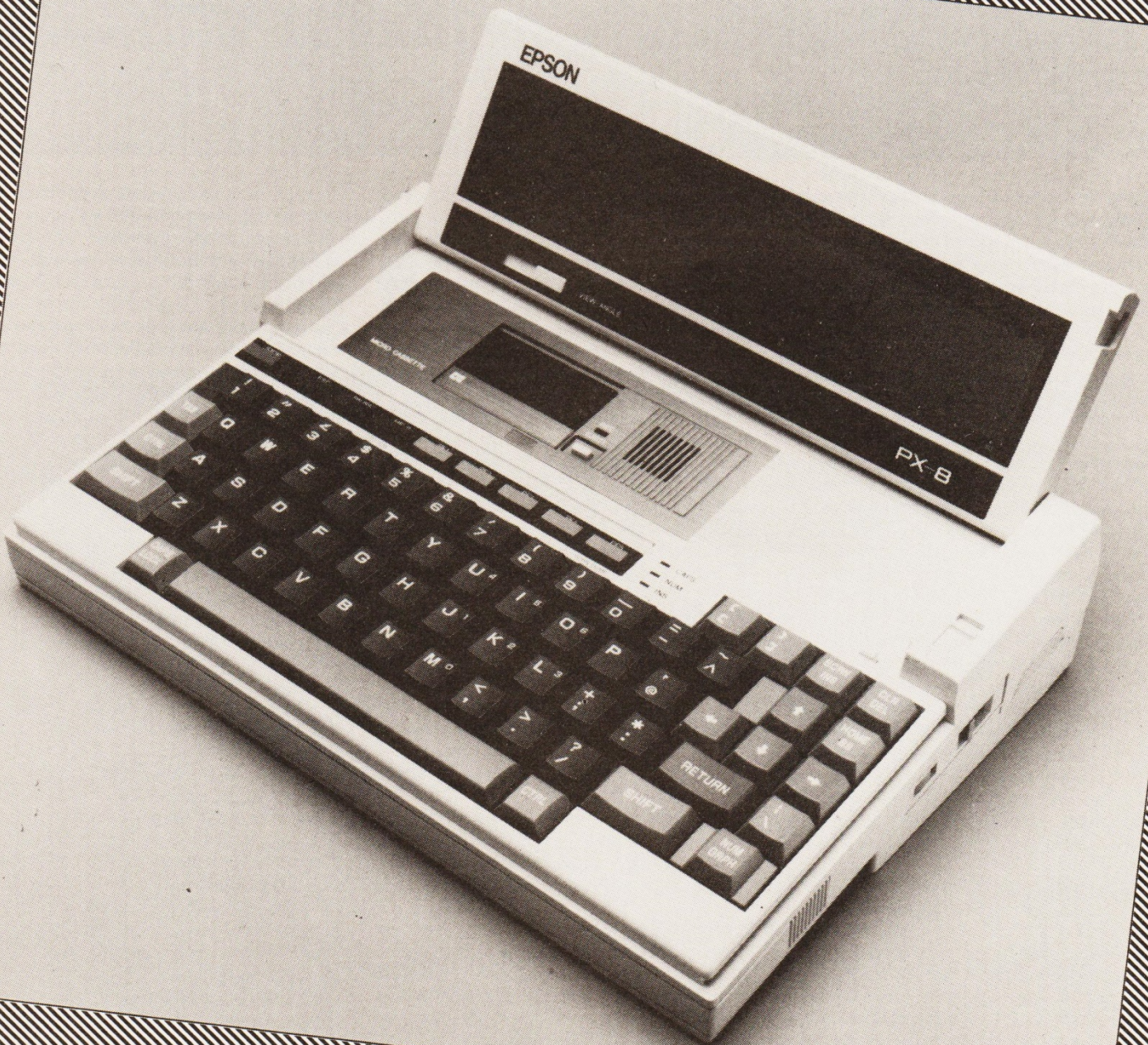
The Epson PX-8 incorporates an 80 character by 8 line LCD screen
